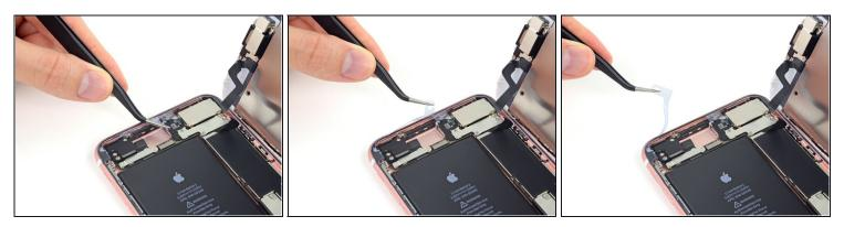
While supporting the display, use tweezers to begin peeling off the final release liners, exposing the adhesive.
