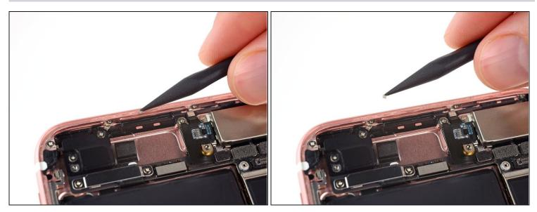
• Use the tip of your spudger to remove any remaining smaller bits of adhesive.
