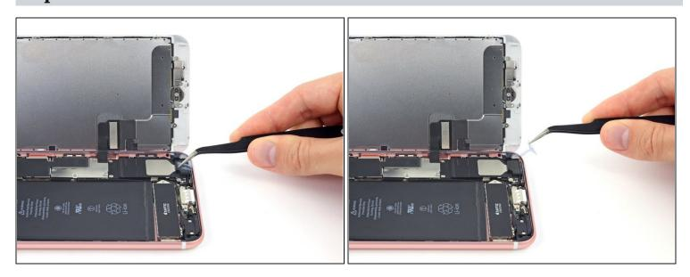
(i) The release liner may consist of two or more pieces. As you remove the final piece, you may need to pause and reposition the display.
