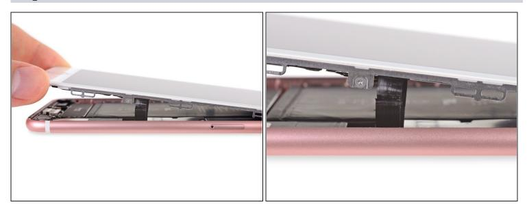
• Before closing up the display, check to make sure that all cables are clear.
