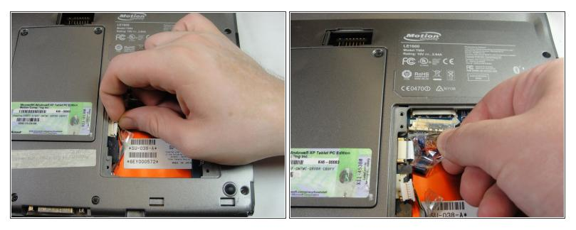
A Caution: do not pull on the wires, instead pull from the plastic connectors.
