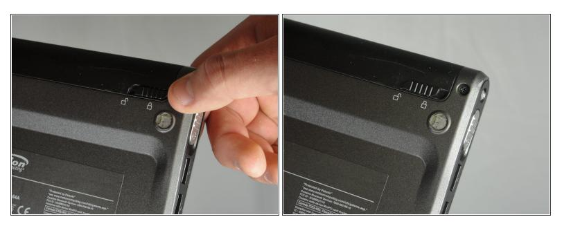
• Slide the battery lock switch next to the power slider to the unlocked position.
