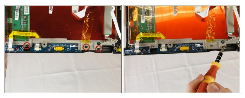
With a Phillips #1 screwdriver, unscrew the three 4mm screws holding the display bracket on the back side of the front buttons.
