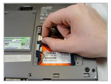
Pull the brown tabs to disconnect the white ribbon cable on the other side.
