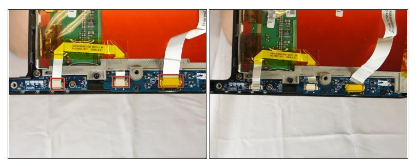
• Unplug the three ribbon cables by pulling on the brown tabs and unplugging cable.
