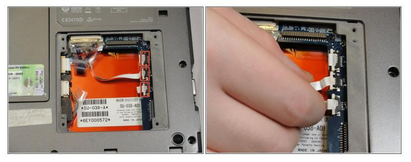
To disconnect the three white ribbon cables on the side closest to the hard drive connector, pull the white plastic tabs.
