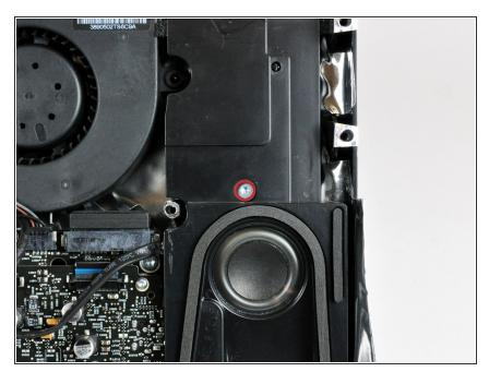
Remove the single T10 Torx screw securing the right speaker to the rear case.
