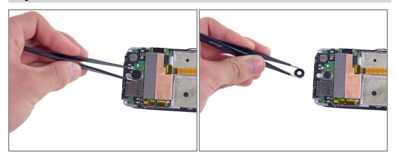
• A camera filter is now free to move, so remove it using <u>tweezers</u>.
