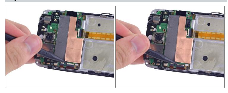
Use the pointed end of a spudger to lift the white tab on the largest ZIF connector opposite the USB connector.
