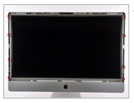
• Remove the eight T10 Torx screws securing the LCD to the outer case.
