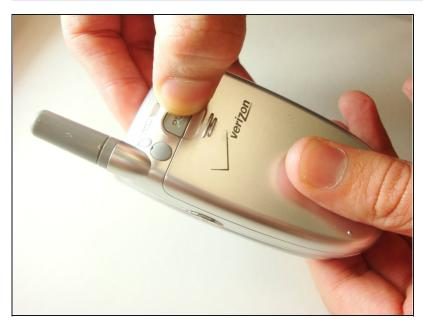
Open the battery casing by pressing the gray "PUSH" button.
