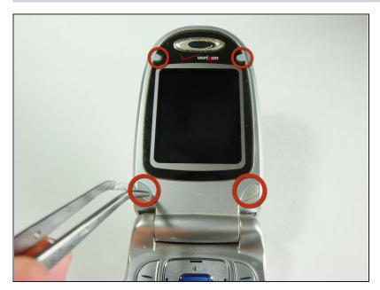
Remove the four grey plugs using either tweezers or a push pin.
