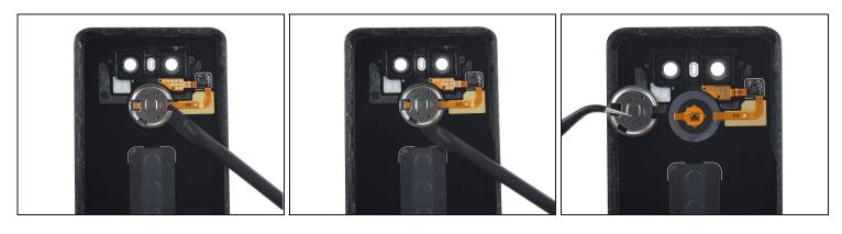
Slide the blade of a halberd spudger into the opening on the edge of the rear button bracket.
