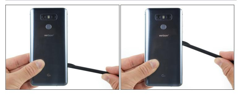
• Slide the blade of a Halberd spudger along the side of the phone, separating the adhesive.
