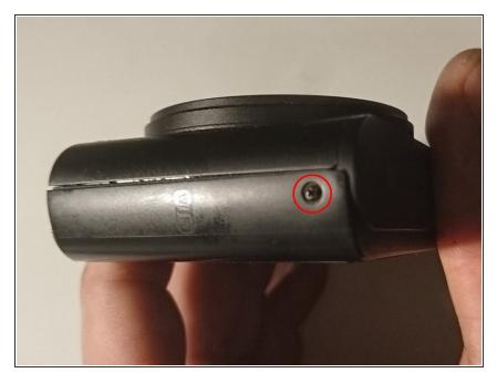
Use the J00 screwdriver to take out the single 3mm black screw on the left side of the camera.
