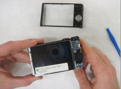
Use the plastic opening tool to pry open the back cover off.
