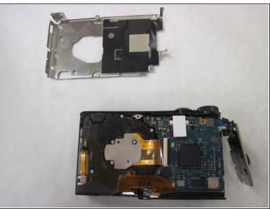
Once the LCD is off use the J00 screwdriver to take out the two 3mm silver screws. Once the screws are taken out pull off the piece with your fingers.
