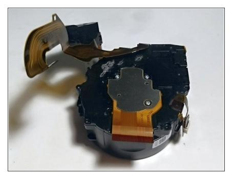
Carefully tear off the ribbon glued to the plastic.
