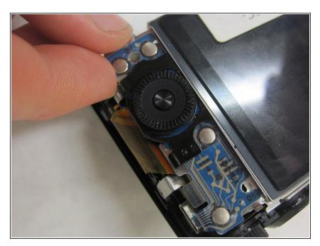
Use your fingers to slide out the controller wheel board 's lower end, then unhook the other end.
