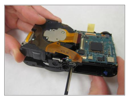
Carefully remove the lens assembly from the camera.
