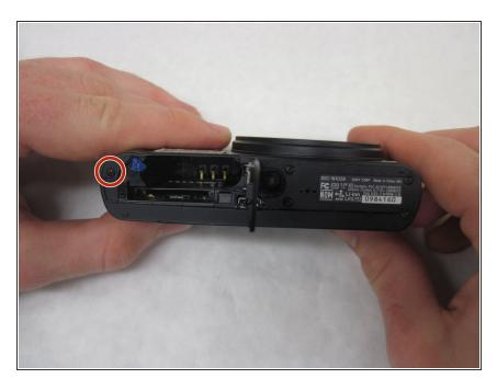
On the bottom of the camera slide the button over to open the battery case. Inside the battery opening use the J00 screwdriver to take out the single 3mm black screw.
