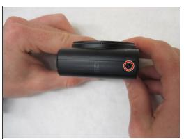
• Use the J00 screwdriver to take out the four 3mm black screws on the bottom and both sides of the camera.
