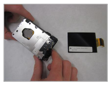
Take the LCD off by undoing the zif and sliding it out.
