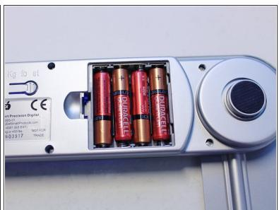
Insert the new batteries in the device.
