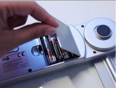
To open the battery compartment, use your finger to gentling push the tip to open the battery compartment.
