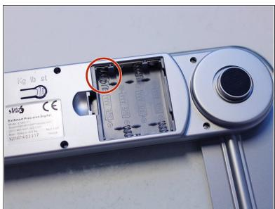
Remove the old batteries from the device by pushing the battery toward the wire side and gentling taking it out.
