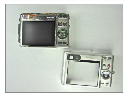
Separate the back case from the body of the camera.
