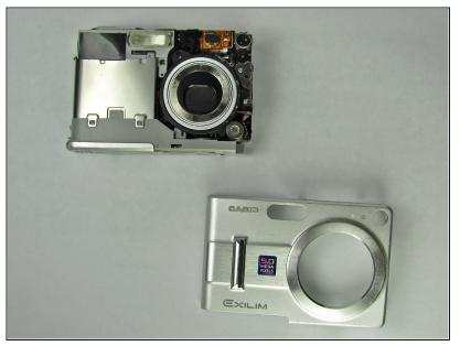
• Separate the front case from the body of the camera.
