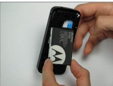
Pinch the sides of the bottom of the battery and pull upward.
