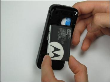
• Pinch the sides of the bottom of the battery and pull upward.
