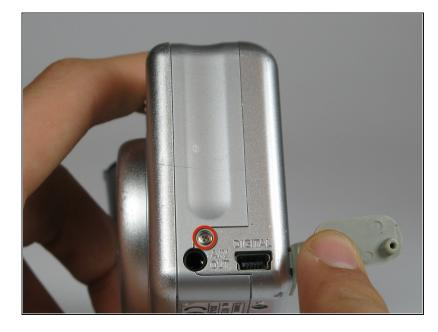
• Remove the 3.8mm screw underneath the flap that covers the A/V port.
