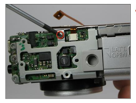
• Remove 2.5mm the screw in the silver housing on the bottom of the camera. This screw is holding the back panel in.
