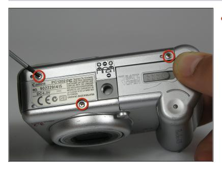
• Remove the three 2.5mm screws on the bottom of the camera.
