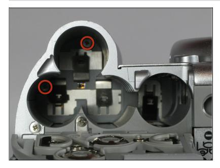
• Remove the two 4.1mm screws at the bottom of the battery flap.
