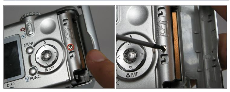
• Remove the 2.4mm screw located underneath the cover of the memory card slot.
