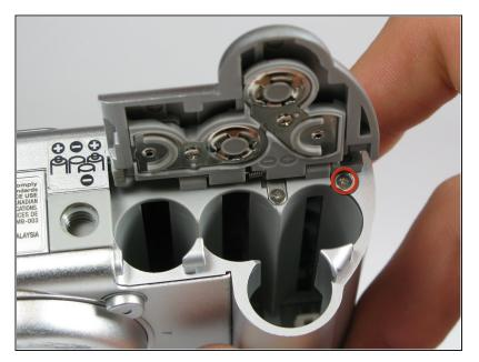
• Remove the rightmost 4.2mm screw underneath the battery cover, not the center screw.
