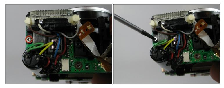
• Remove the 3.5mm screw found near the capacitor and the flash unit.
