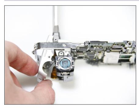
Carefully remove the other side of the lens casing by pulling it away from the lens, and make sure to keep attached to the wire it is connected to.
