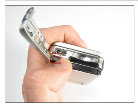
Push the small gray plastic tab away from the battery in order to release the battery.
