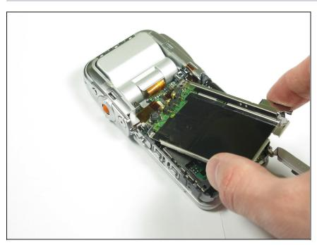
Carefully remove the motherboard from the camera by grasping the sides and pulling upwards and then outwards.
