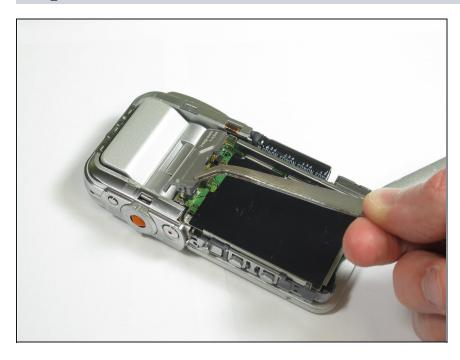
Remove the small cover from near the top of the motherboard, using tweezers or forceps, as in the picture.
