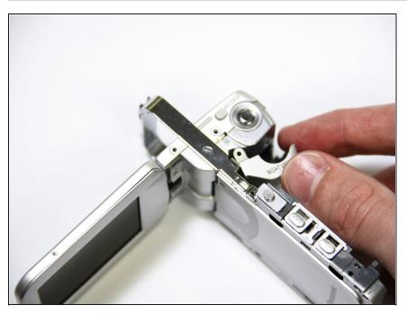
Carefully remove the bottom of the lens casing by pulling downwards away from the lens.
