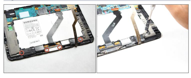
• Using a Phillips #00 screwdriver, unscrew the 4 screws (3mm) that are holding the charger port and speaker support.
