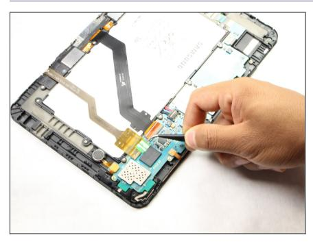
• Using <u>tweezers</u>, peel away the green tape located on top of the two flexible ribbon cables.
