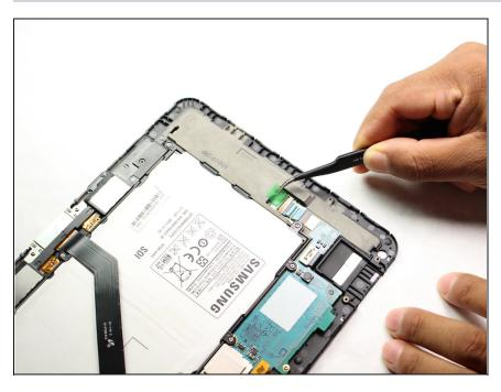
• Remove green tape from lcd connector.
