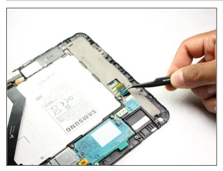
• Pull lcd cable out of connector.
