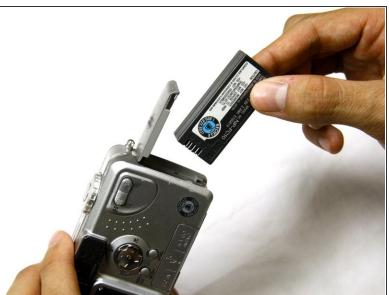
Remove the battery from the camera.
