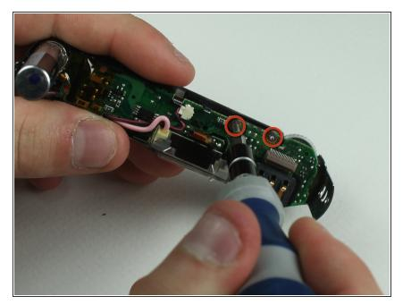
Unscrew the small screws beneath the top cover(#00P, 1.7mm).
