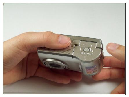
• Locate the battery compartment on the bottom right of the camera.
