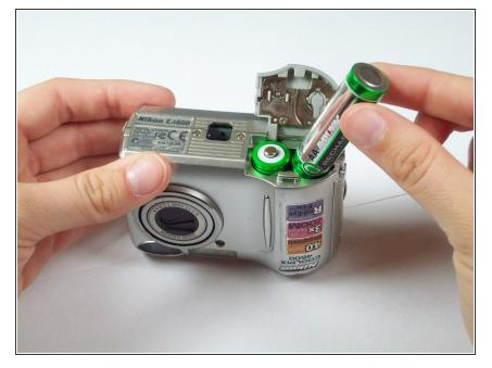
Remove the dead batteries. The easiest way to do this is by turning the camera right side up and gently tapping the lens side of the camera against your hand until they fall out. If this does not work, you can simply pull them out.
