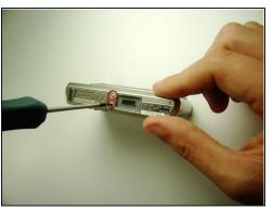
• Locate and remove the 3mm screws on the bottom and sides of the camera with a JIS size #0 screwdriver.
