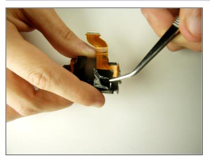
With the <u>tweezers</u> remove the black tape to detach the chip from the lens box.
