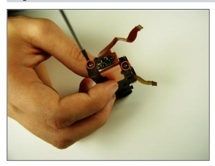
Locate and unscrew the two 3mm screws on the bottom of the black lens box with the JIS #0 screwdriver.
