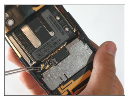
Use tweezers to remove the DIV and GPS antennas from the back of the keyboard.
