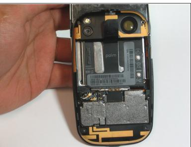
Use the t4 screwdriver to remove all 6 of the 3.6mm long screws.
