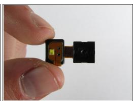
With two fingers carefully detach the camera from the motherboard by lifting straight up.
