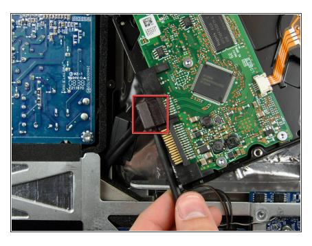
Disconnect the SATA data cable by pulling its connector away from the hard drive.
