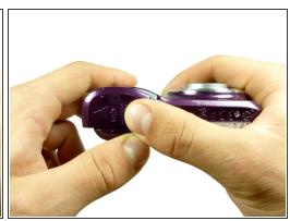
First, access the slide door on the bottom left corner of the camera. To open, push down and to the left.
