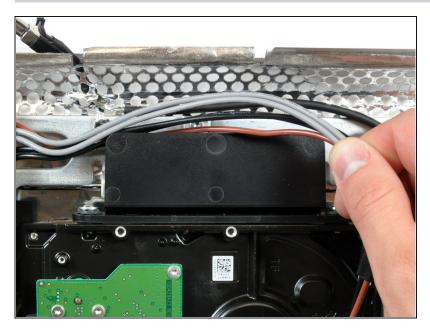
• De-route the bundle of power supply cables from behind the hard drive bracket.
