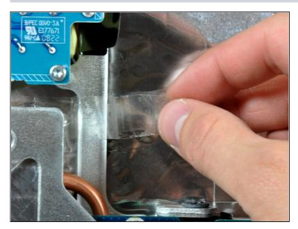
(i) If necessary, remove the piece of tape holding the AC-in cable under the chassis.
