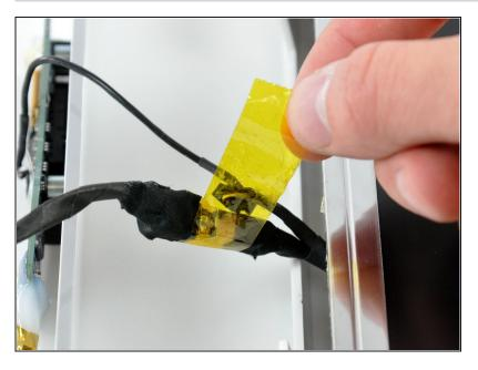
If necessary, remove the piece of kapton tape(it is ok to toss this) wrapped around the microphone and camera cables.
