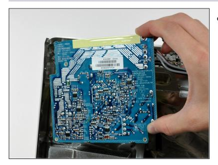
• Lift the power supply out of the rear case, minding the AC inlet cable that may get caught on the chassis.
