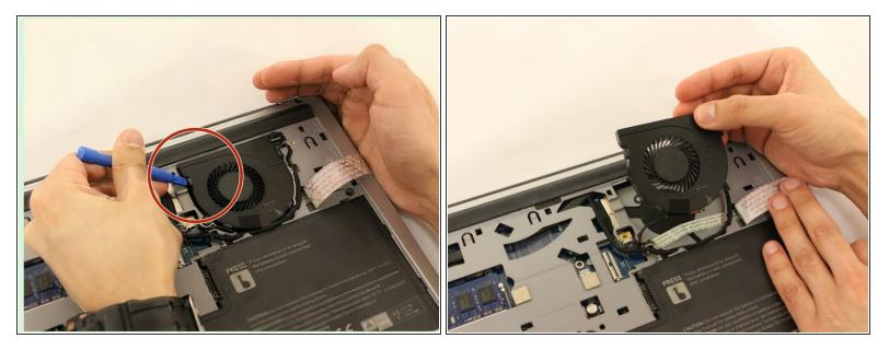
• Using the opening tool, pry the fan out.
