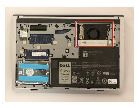
• Locate the fan system in the top right corner.
