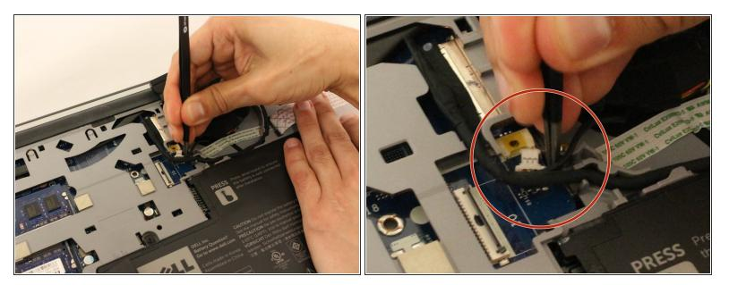
• Use tweezers to remove the small cable attached to the fan.
