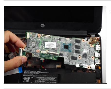
Gently slide the motherboard to the left and away from the external ports on the right and then pull it up and out of the laptop.
