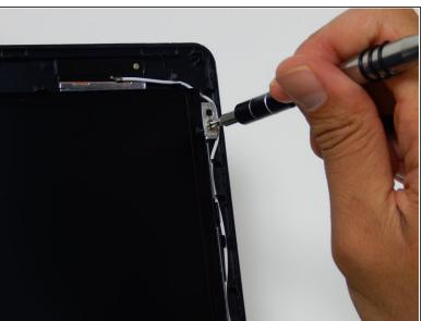
Remove the six 3.35mm screws with a Phillips #0 Screwdriver.
