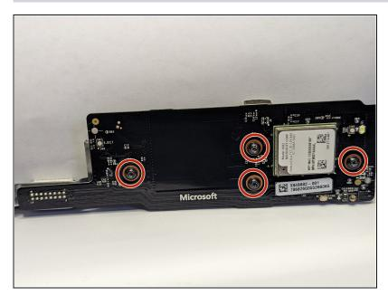
Remove the four black 8 mm T-9 Torx screws labeled "E1," "E2," "E3," and "E4."
