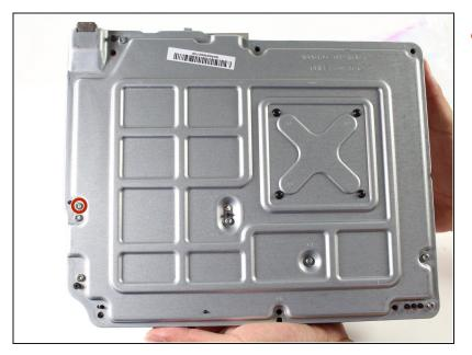
To remove the optical disc drive, remove the silver 10 mm T-10 Torx screw labeled "C4."
