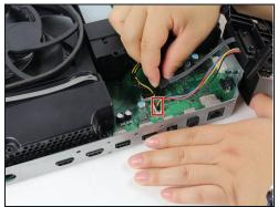
Gently disconnect the hard drive from the motherboard (at the two plastic connector bodies).
