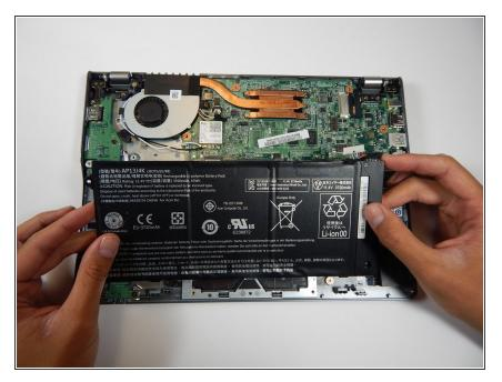
Lift the battery from the frame.
