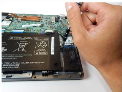
• Remove the the two 3.7 mm screws with a Phillips #0 screwdriver.
