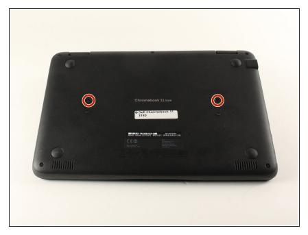
Using tweezers, remove the circular stickers that are covering the two screws near the middle of the back cover. Stick them to the laptop next to the screws.
