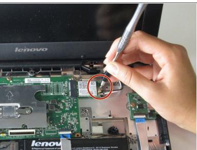
Use a screwdriver to remove the single 3mm Phillips screw that is holding the WiFi card in place.
