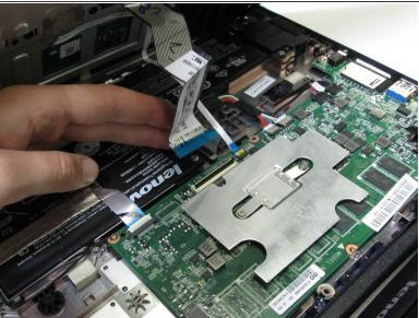
Disconnect the keyboard ribbon cable by lifting the ZIF connector lock with a plastic opening tool or fingernail and gently pulling the ribbon cable straight out of its socket.
