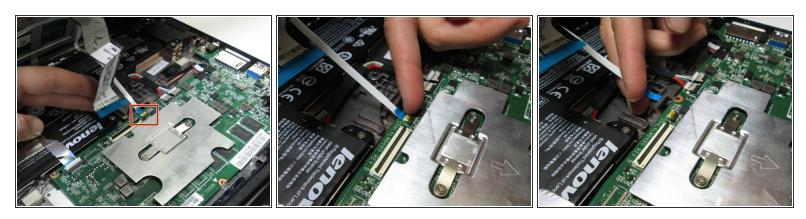
Disconnect the trackpad ribbon cable by lifting the ZIF connector lock with a small prying tool or fingernail and gently pulling the ribbon cable straight out of its socket.
