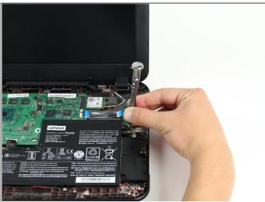
Use a Philips #1 screwdriver to remove the three 4.3 mm screws securing the battery.
