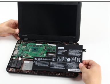
Lift up on the tabs that were held down by the screws to remove the battery.
