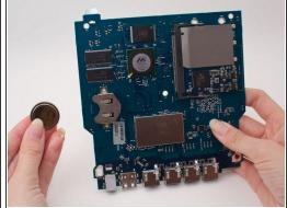
Remove the battery by gently "shoving" it out with the plastic tool.
