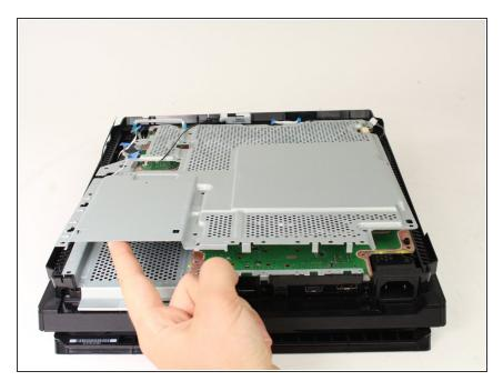
Pull up and remove the metal plate.
