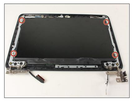
Using a Phillips #0 screwdriver, remove all four silver 3mm
