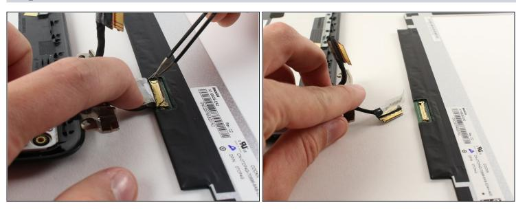
• To unplug the screen, use tweezers to lift the small metal wire on the connector, and then gently pull the cable away from the screen.
