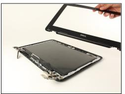
• Using a plastic opening tool to start, and then eventually your hands, pry the front most face of plastic off of the screen assembly.
