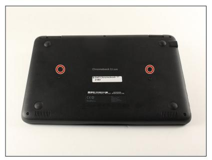
Using tweezers, remove the circular stickers that are covering the two screws near the middle of the back cover. Stick them to the laptop next to the screws.
