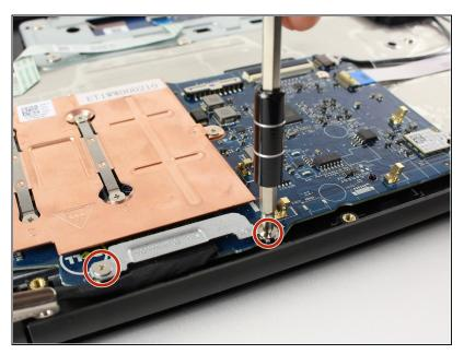
Using a Phillips #0 screwdriver, remove the two 3mm Phillips head screws from the metal bracket that covers where the wrapped cable from the screen attaches to the motherboard.
