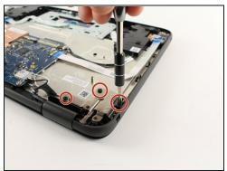
Using a Phillips #0 screwdriver, remove each of the five 5.5mm screws.
