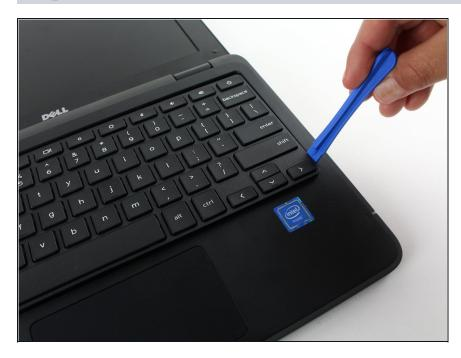
Remove the keyboard from the body. To do this, use a plastic prying tool to get under the keyboard and pry it up from the computer body.
