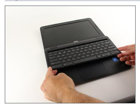
• Once you have separated the keyboard and the body using a spudger or plastic opening tool, use your hands to pull it away from and off of the computer.
