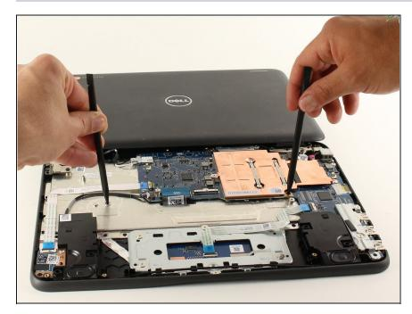
Release the keyboard from the body. To do this, push on the two keyboard release holes with something thin and cylindrical like a spudger or a pencil. Step 8
