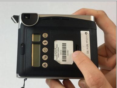
• The battery compartment can be found on the backside of the camera. Pinpoint this compartment and focus on the right edge of the compartment gate to find the opening latch.
