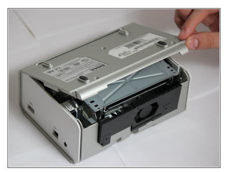
Rotate the photo printer so that the bottom panel faces up once again.
