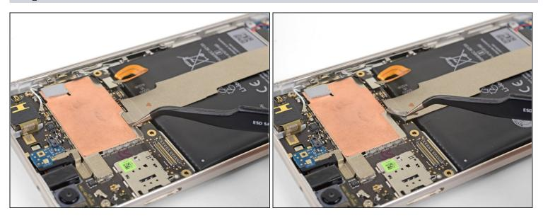
• Use <u>tweezers</u> to peel up the tape at the top of the interconnect cable.
