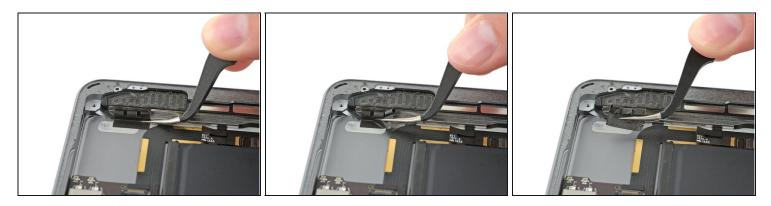
• Carefully peel the LCD buffer tape up off of the rear case.
