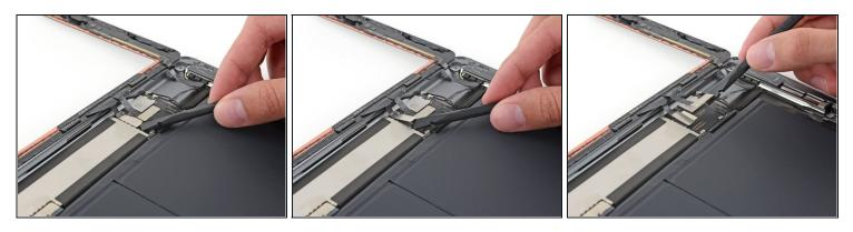
• Use a the flat end of a spudger or a fingernail to carefully pop the two digitizer cable connectors straight up from their sockets.
