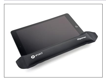
Heat an iOpener and apply it to the left edge of the device for two minutes.
