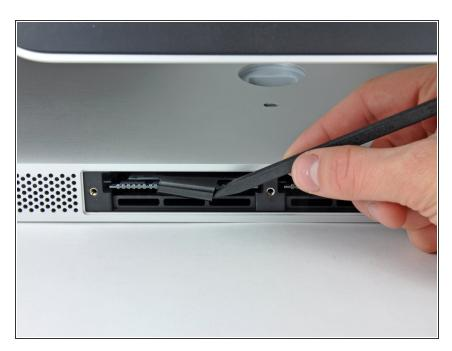
Use your fingers or the tip of a spudger to slide the black plastic RAM tray pull tab out of the RAM slot.
