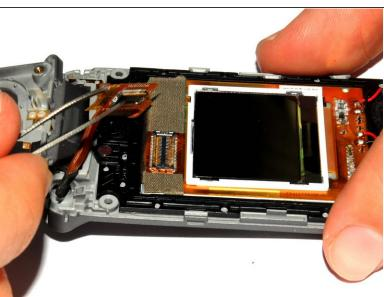
Use the tweezers to lift the display adapter off the screen component.
