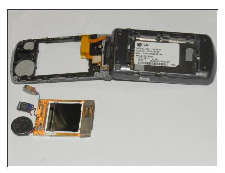
Lift the screen components out of the phone.
