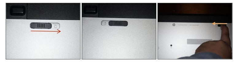
• Once the computer is off, remove the battery. Switch the locking tab to the unlocked position.
