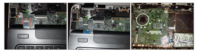
With the keyboard and trackpad disconnected, disconnect the power button. Flip the black tab up and remove the palmrest.
