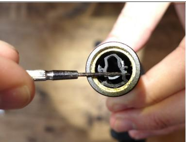
Rubber band is irreparable and needs to go. I scratched it out using a small, sharp screwdriver.
