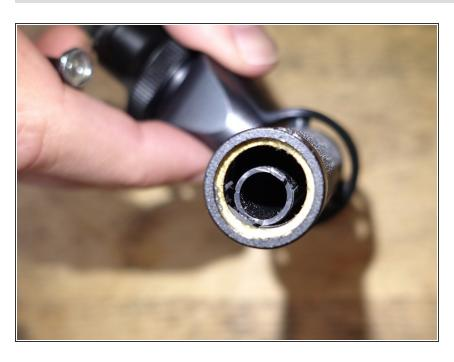
The culprit of the rattling noise is now apparent. A plastic cylinder stretches through the whole of the
