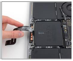
Carefully peel the trackpad ribbon cable up off the battery, and push it out of the way.
