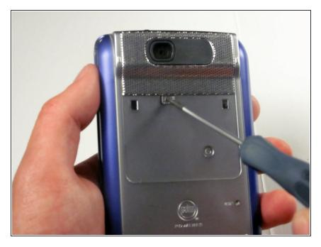
Use a #00 Philips screwdriver to remove the 2.5mm hidden screw.
