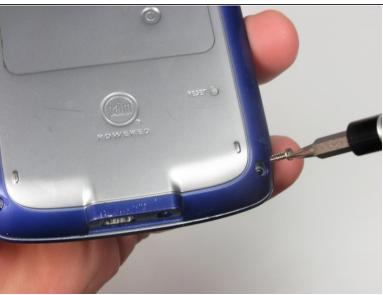
Using a T5 Torx screwdriver, unscrew the two 5mm screws located at the bottom of the device.
