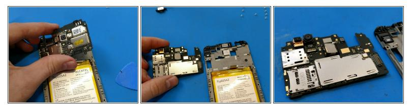
• A quick discount of the daughter board flex and antenna cable releases the board from the mid frame.
