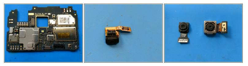
• We have the board out, time to take the proximity sensor, front facing 5MP camera, and rear facing 8MP camera out. All are simple modular parts.
