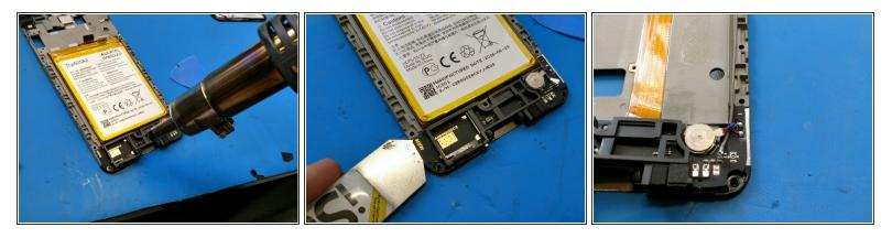
• A wee bit of heat to melt the adhesive, and the daughter board is almost out, looks like we need to take the battery out first.
