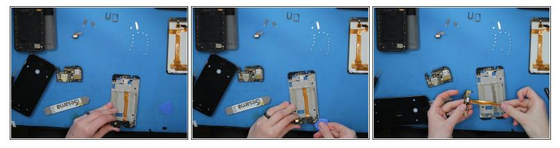
• Some careful lifting of the board and the flex cable gets the board off the mid frame.
