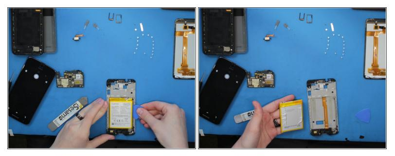
• A simple prying to the battery with a plastic pick gets it right out. Remember to use plastic, we don't need a Note 7 here.
