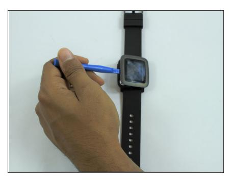
• Carefully, pull apart the cover with the plastic opening tool.
