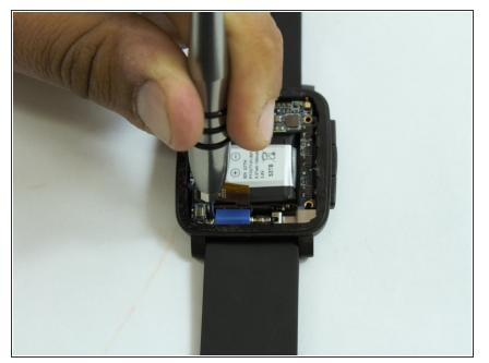
• Remove the final screw from the circuit board with a J000 Philips head screwdriver.
