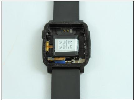
After removing the circuit board, the battery is located in the middle of the case.
