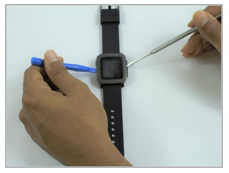
• Use the metal spudger tool to carefully loosen the rest of the cover.
