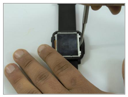
• Insert metal spudger into the side of the screen shown in the picture.
